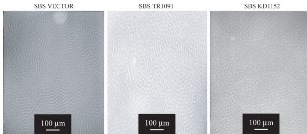
Figure 16 TEM photomicrographs of each type of SBS (VECTOR, KD1152 and TR1091) in PBT/SBS 70/30 blends extruded at 220°C and injection molded at 240°C. [Color figure can be viewed in the online issue, which is available at www.interscience.wiley.com .]
